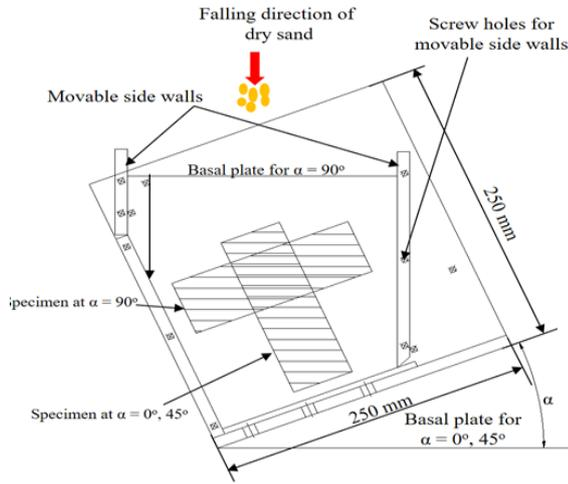
Figure 3: Container with movable walls
