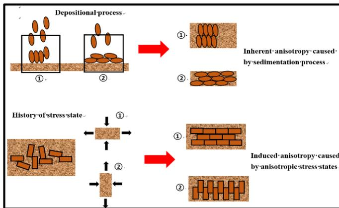
Figure 1: Definition of two types of anisotropy
