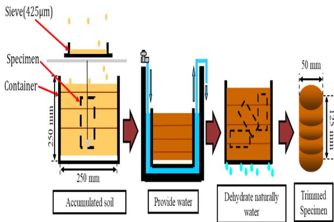
Figure 4: Process of making the specimen
